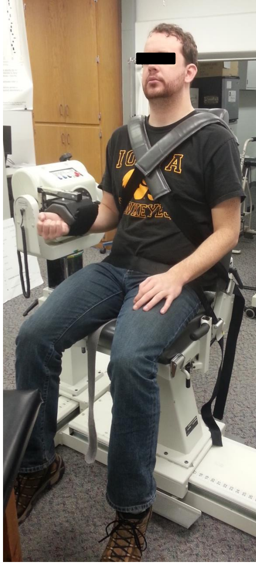
Figure 1- 2: A controlled isometric fatiguing bicep curl task using a constant angle.
